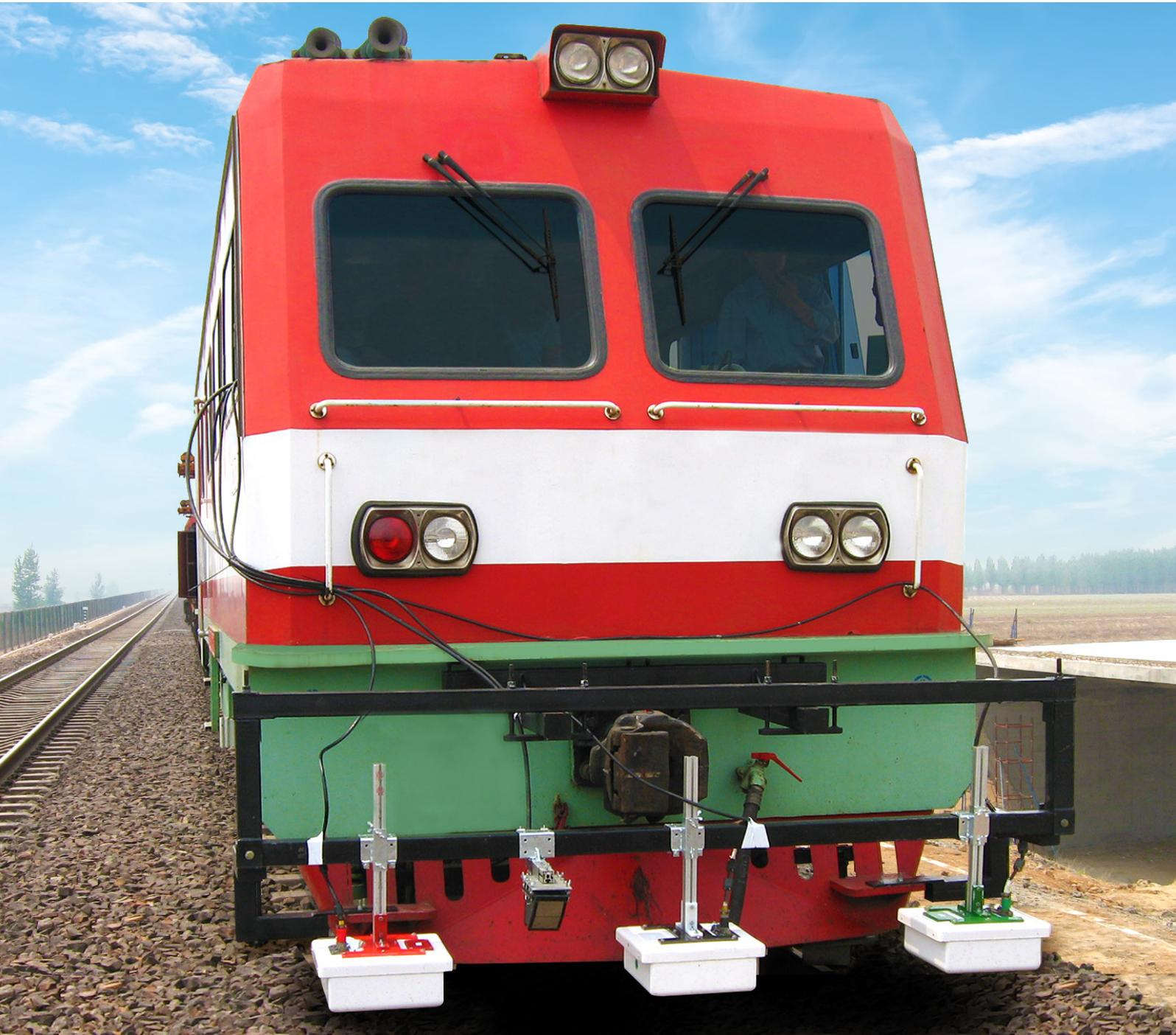
The integrated solution for autonomous railway ballast inspection with a high acquisition speed, fast processing and automatic data interpretation
