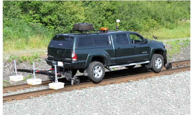
Road-rail vehicle equipped with SRS
