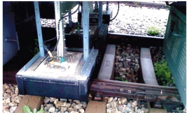
SRS configured with antennas beneath the train
